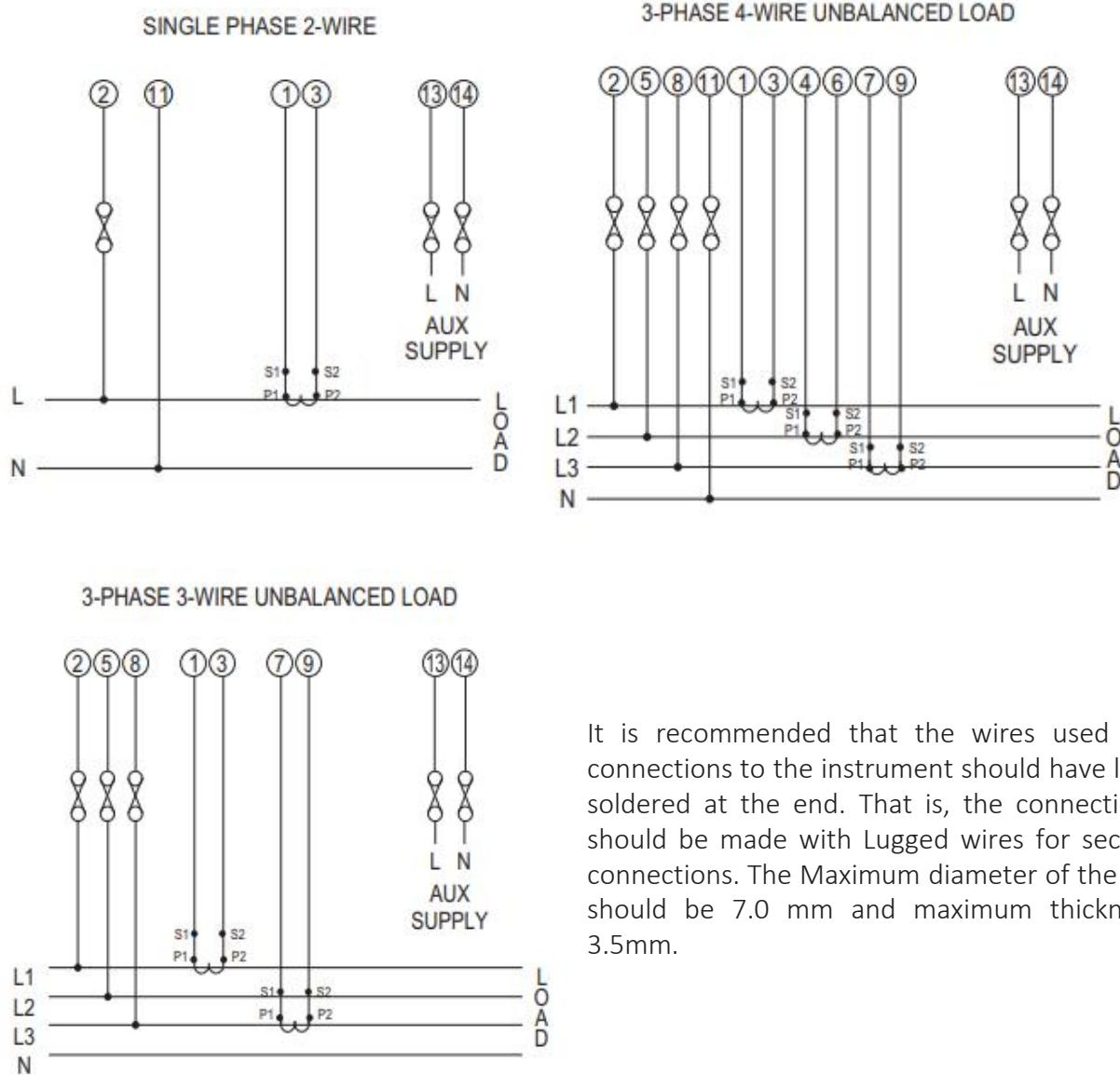
It is recommended that the wires used for connections to the instrument should have lugs soldered at the end. That is, the connections should be made with Lugged wires for secure connections. The Maximum diameter of the lug should be 7.0 mm and maximum thickness 3.5mm.
