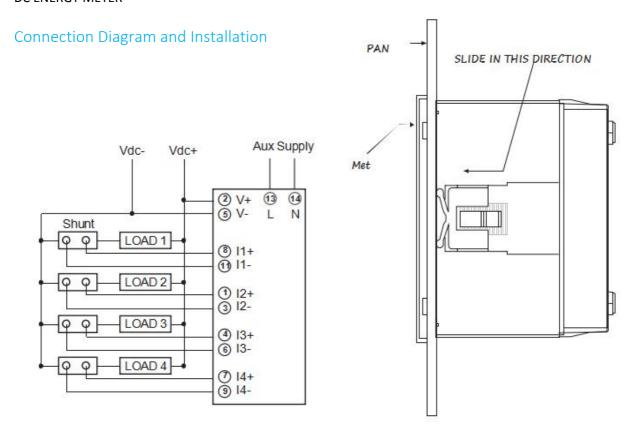
It is recommended that the wires used for connections to the instrument should have lugs soldered at the end. That is, the  $connections \ should \ be \ made \ with \ Lugged \ wires for secure \ connections. \ The \ Maximum \ diameter \ of \ the \ lug \ should \ be \ 7.0 \ mm \ and$ maximum thickness 3.5mm. Permissible cross section of the connections wires: <= 4.0 mm sqr. single wire or 2x2.5mm sqr. fine
