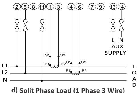
It is recommended that the wires used for connections to the instrument should have lugs crimped at the end. That is, the connections should be made with Lugged wires for secure connections.
