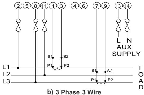
**Note :** L2 phase needs to be connected in terminal 11 instead of terminal 5 only for 3 Phase 3 Wire connections.
