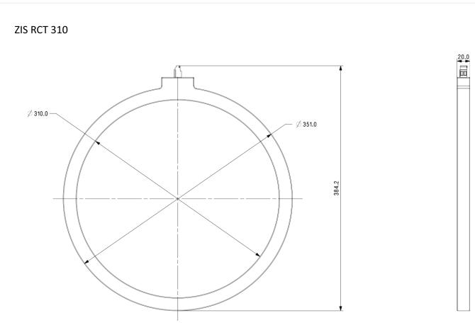
Note : The above given RCT comes with a tape winding and not in Plastic Case.
